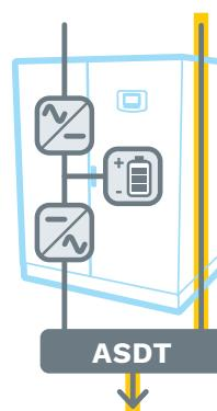
*In the event of power supply failure the internal automatic device (ATSD) transfers the load to the inverter. The battery provides power to the inverter, ensuring the required runtime.*
