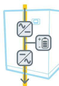
*the event of power supply failure the battery provides power to the inverter, ensuring the required runtime with no interruptions at all.*
